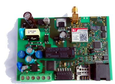
The remote control unit is a high performance, high reliability board for control of industrial processes and installations. It has many communication ports for connection to other equipment.
